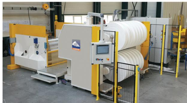
*For example, answering a specific customer need, we engineered around our cutting-edge unwinding / slitting / rewinding technologies, a 3 axles non-stop turret winder with loading from floor, printing, slitting and cross cutting, coreless rewinding, labelling and automatic unloading". This development has been made possible thanks to the support of Calemard's integrated engineering department and its well-equipped testing shop.*
