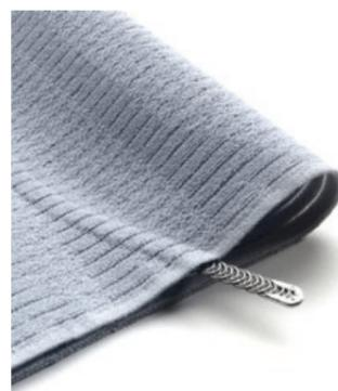
To address the wide variety of body shapes, no less than eight sizes of back belts are currently required on the market, imposing significant stock requirements on pharmacists, and therefore, considerable costs. By developing a gripping elastic fabric through weaving, Berthéas offers a cost-effective solution. With
